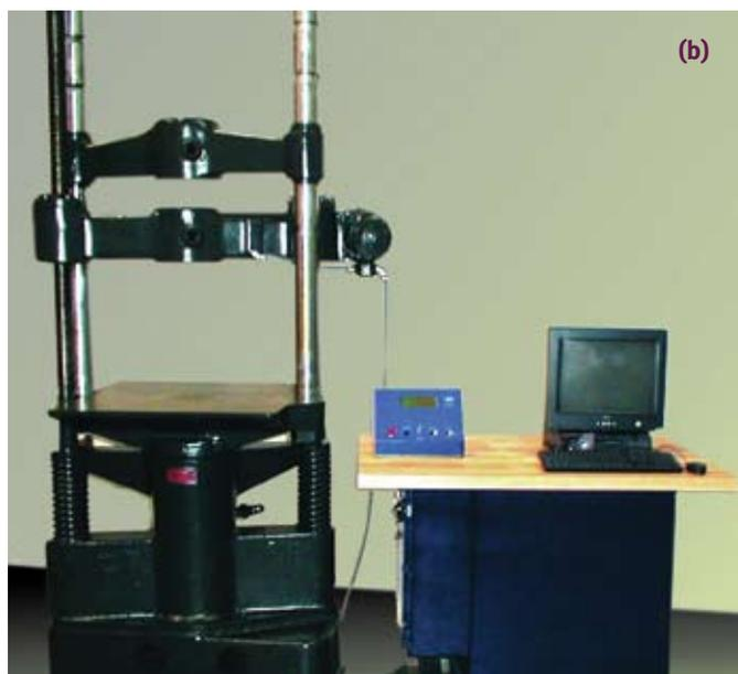
**Fig. 2: The MegaForce II system can also be used in conjunction with the MTESTWindows system to retrofit existing universal testing machines: (a) a Baldwin 270 kN (60 kip) universal testing machine with the original manual controls; and (b) a similar testing machine retrofitted with the MTESTWindows system**
