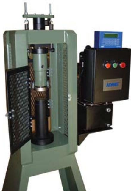
**Fig. 1: ADMET MegaForce II system mounted on a concrete compression testing machine for breaking concrete cylinders, prisms, and beams**
