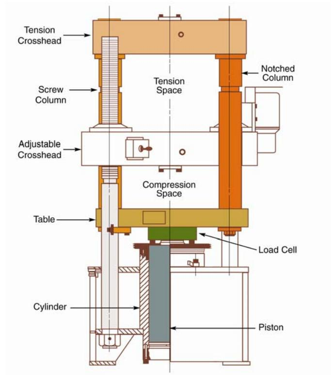
Figure 2: Anatomy of a universal hydraulic testing machine.
